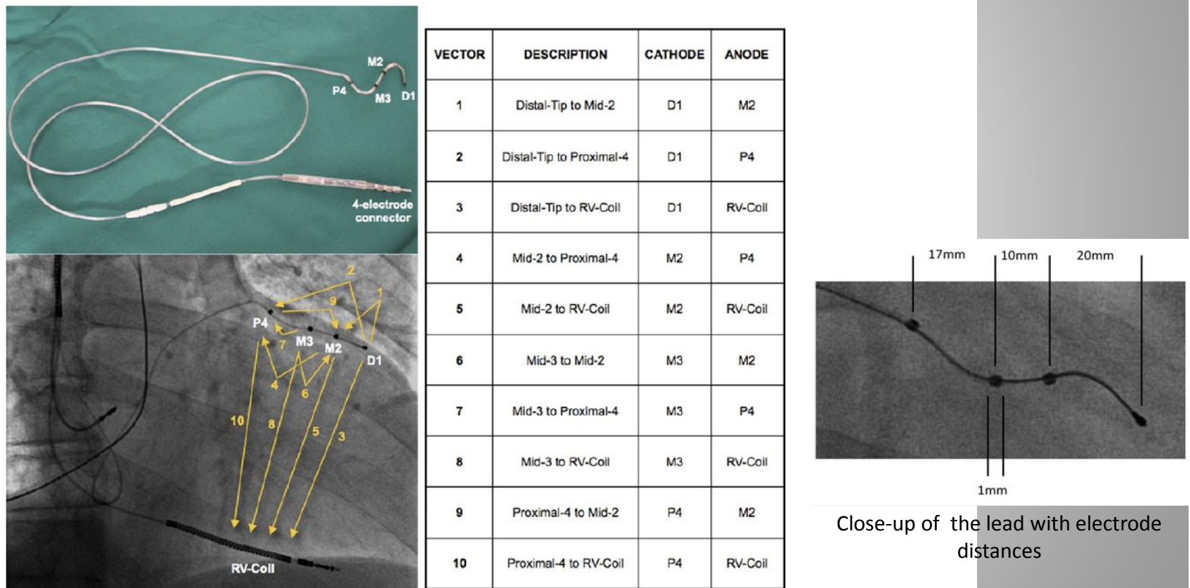
Figure 1 View of the quadripolar left ventricular lead with a detailed representation of the multiple pacing vectors. The 3-ring electrodes (M2, M3, P4) are located 20, 30, and 47 mm from the 4.0-F-tip electrode (D1). Maximum lead body diameter is 4.7-F. In conjunction with an appropriate device, it enables delivery of pacing stimuli using any of the 4 electrodes in 10 pacing configurations. Bottom: final lead location at implantation from the right anterior oblique projection. RV = right ventricular.
